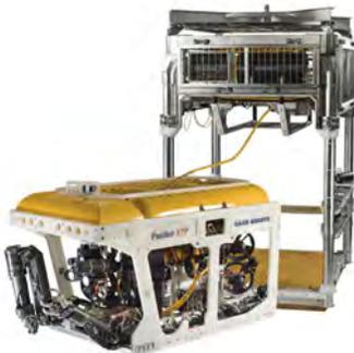
The Seaeeye stainless steel TMS type 8 uses a bail arm to spool up to 200m of tether on and off a drum controlled by the ROV pilot. The TMS height can be adjusted to accommodate different tool skids.
