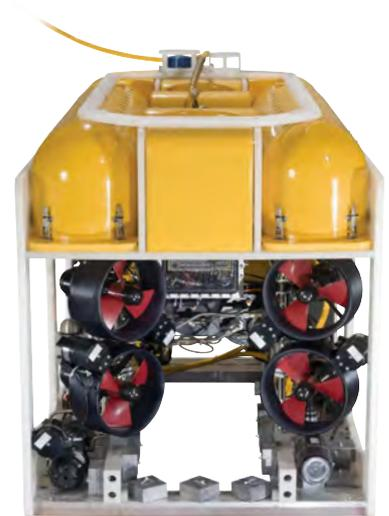
PANTHER-XT PLUS SHOWING TOOL SLEDGE COMPARTMENT
