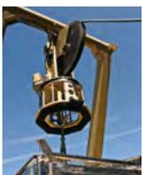
A snubber-rotator assembly allows the TMS to be locked into position and rotated for a safe and smooth transit through the A-frame (optional).
